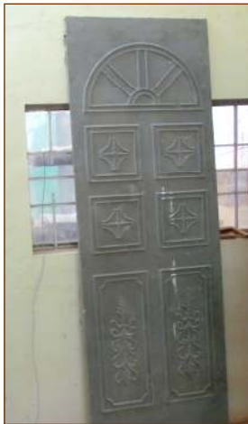
Ferrocement door made by Dr. Jagannath at Podicherry engineering College, India
